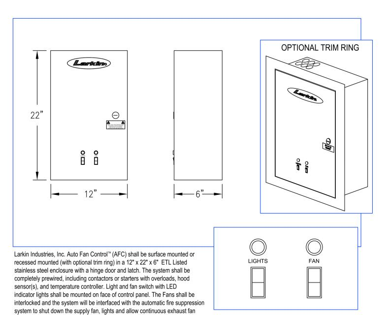
operation during fire. The Auto Fan Control ™will automatically energize the fan(s) and light(s) as the temperature of the cooking equipment rises prior to cooking operations commencing in compliance with IMC 507.1.1. System shall include a "cool down" delay that allows fans to operate for approximately 30 minutes after cooking equipment has been turned-off and an additional rise in temperature has not been detected.
