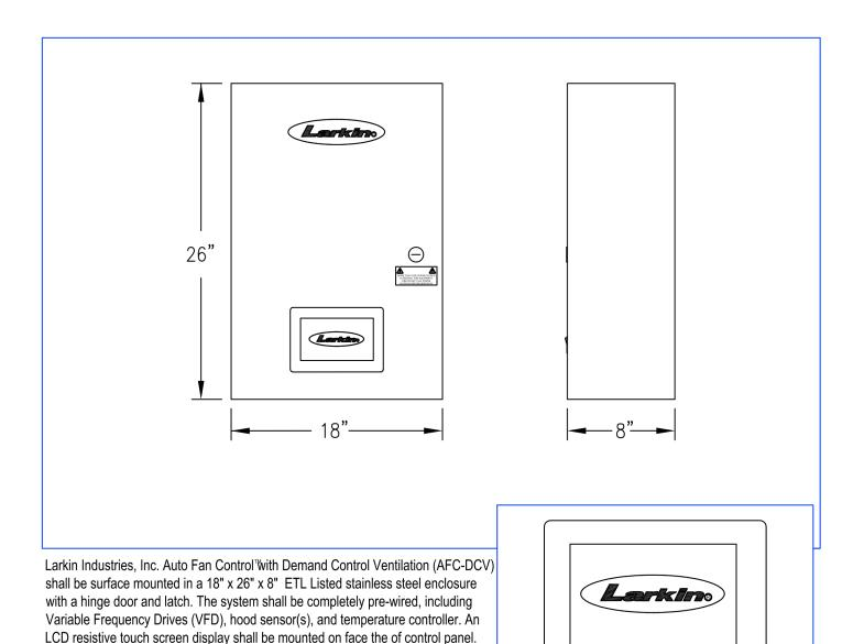
the fan(s) and light(s) as the temperature of the cooking equipment rises prior to cooking operations commencing in compliance with IMC 507.1.1 and will modulate fans based on cooking load and building pressure. System shall include a "cool down" delay that allows fans to operate for approximately 30 minutes after cooking equipment has been turned-off and an additional rise in temperature has not been detected.
